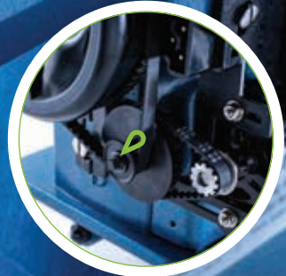
33 Right end lubrication points
