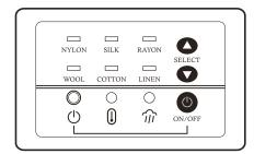
**IMPORTANT NOTE:** If you can not determine the type of fabric, begin with the lowest setting and increase the temperature as desired until you obtain the proper results.
